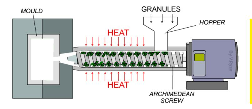
GRANULES OF POLYPROPYLENE ARE ADDED TO THE HOPPER.
