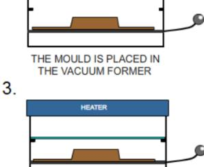
PLASTIC SHEET IS PLACED ABOVE THE MOULD AND CLAMPED SECURELY.
