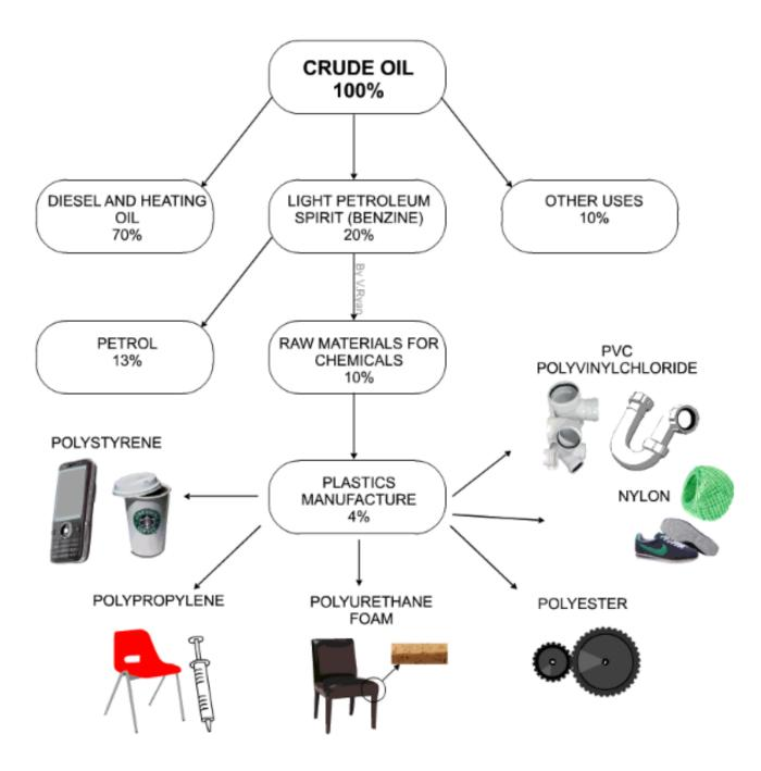
The diagram below outlines the processing of crude oil and its subsequent use as fuels, oils, gases and plastic products.
