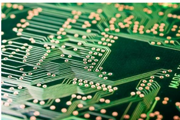
Printed circuit boards are made when copper sheets are etched using iron(III) chloride solution. Where the copper has been etched, only plastic remains.
