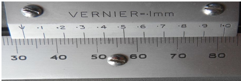
Figure 2 - Vernier scale reading 32.4 mm
