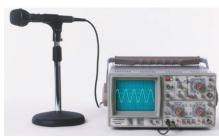
An oscilloscope is a piece of equipment which can help us visualise sound waves.
