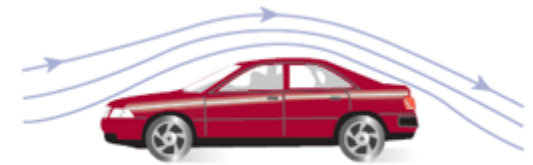
The air flow over a car travelling at low speed
