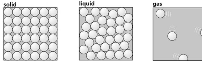
Solids usually have a higher **density** than liquids or gases because they contain more **particles** in a certain volume, the **particles** are therefore closer together. Gases can be compressed (squashed) because there is space between the **particles**.
