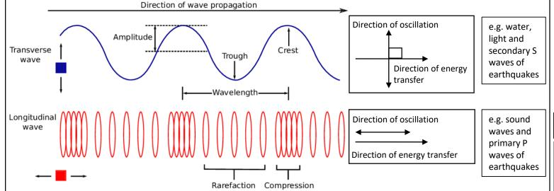
For a transverse wave the direction of oscillation is perpendicular to the direction of energy transfer, whereas for a longitudinal
