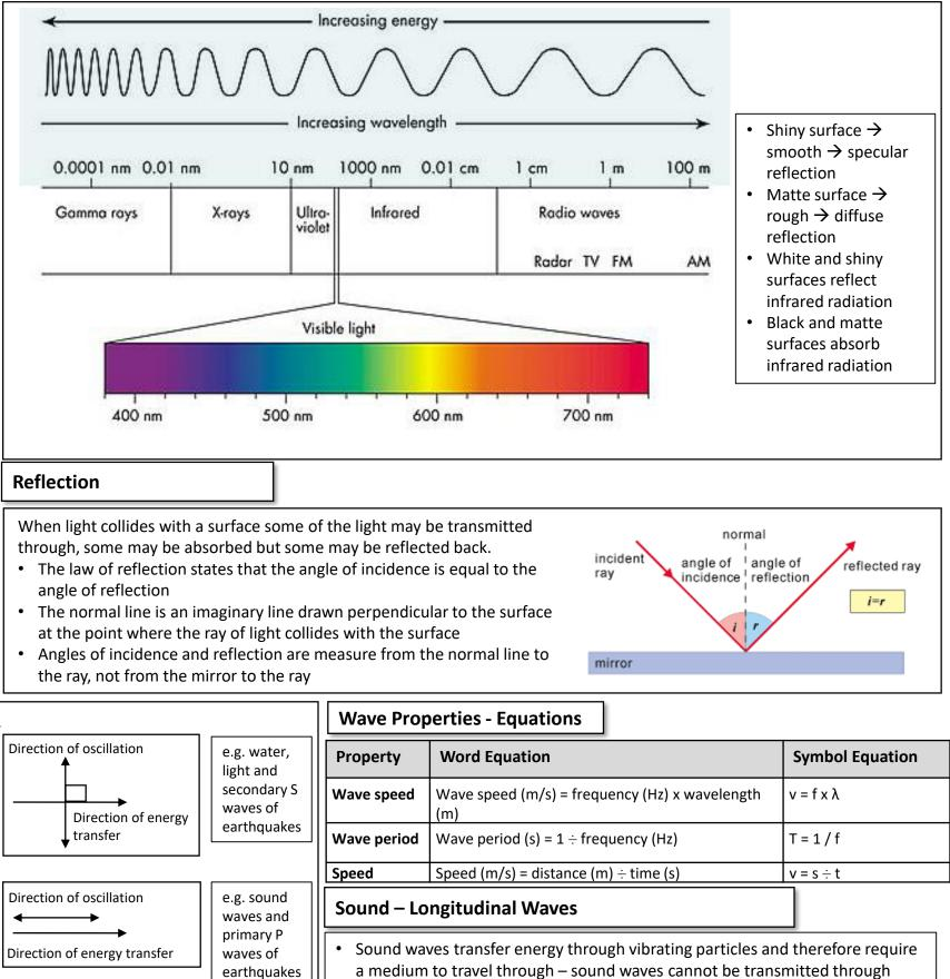
For a transverse wave the direction of oscillation is perpendicular to the direction of energy transfer, whereas for a longitudinal wave the direction of oscillation is parallel to the direction of energy transfer
