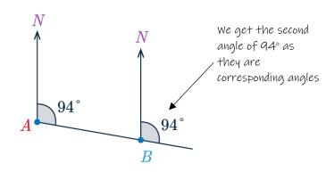
If we know the bearing of B from A is  $94^{\circ}$  then we can calculate the bearing of A from B by extending the line between the points.
