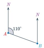
In this example we would say the bearing of B from A is  $110^{\circ}$  rather than the bearing from A to B is  $110^{\circ}$ .
