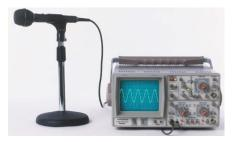
An oscilloscope is a piece of equipment which can help us visualise sound waves. Sound waves cannot usually be seen when they are transferred through a material. However, using a microphone and an oscilloscope, we can transform the longitudinal sound wave into a transverse wave that can be seen on the oscilloscope screen.
