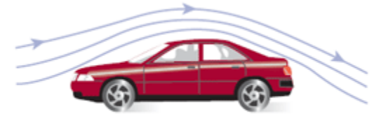
The air flow over a car travelling at low speed
