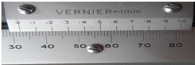
Figure 2 - Vernier scale reading 32.4 mm
